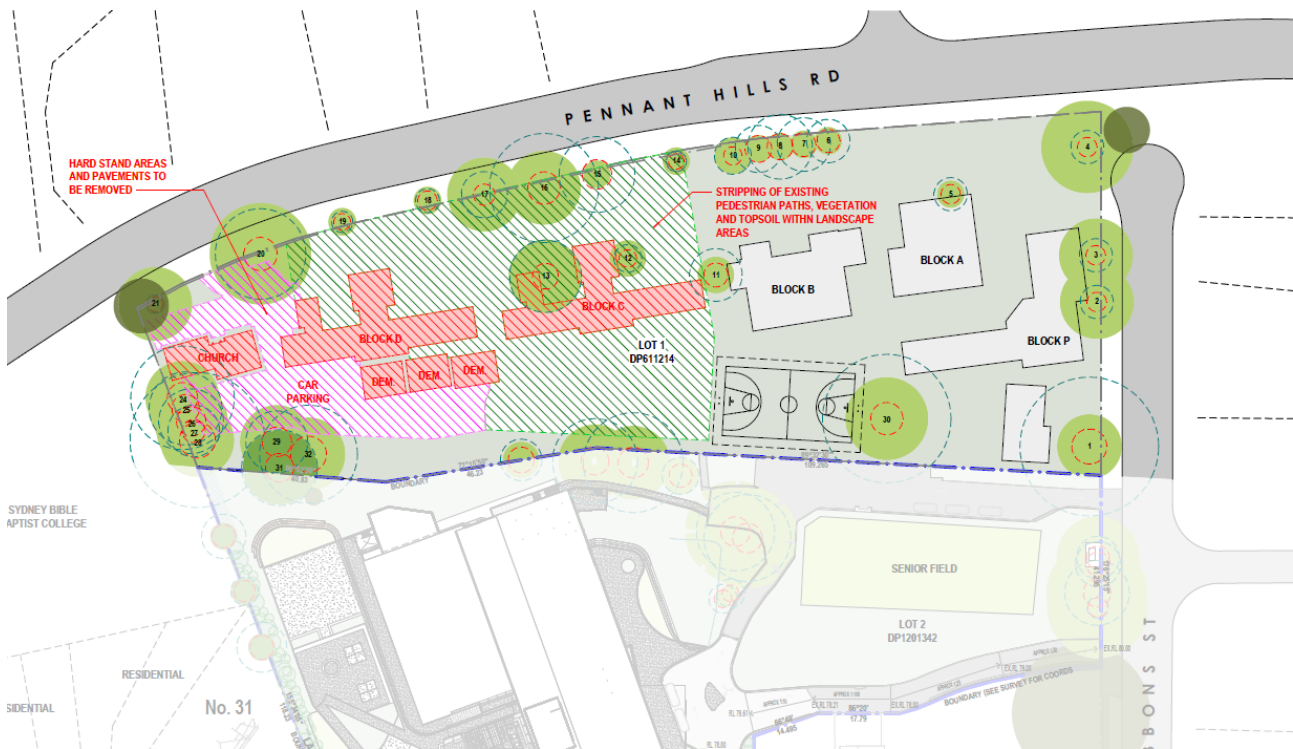
Figure 4: Demolition Schedule (source: Leaf Architecture, 2024))
